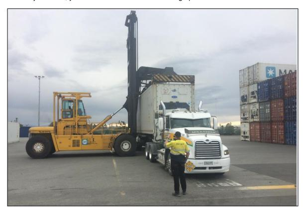
8 If uplifting a container, when the load is complete and the container is correctly sitting over the truck's twistlocks, give the "thumbs up" to the top lifter driver, to signal the load is successful.
